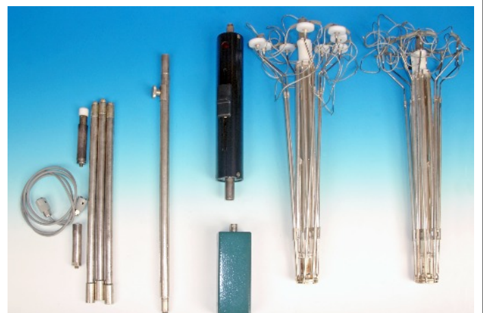
Complete 'Umbrella' aerial kit in canvas transport cover (left) and shown in individual parts (right). The blue block fitted with a BNC socket in the centre below the variometer was a low pass filter which clipped at the right hand side of the WSA 1 transmitter in place of the aerial tuning unit.
