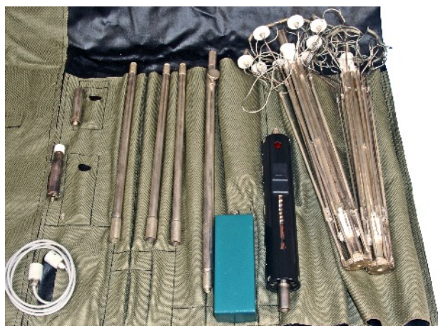
Complete 'Umbrella' aerial kit in canvas transport cover (left) and shown in individual parts (right). The blue block fitted with a BNC socket in the centre below the variometer was a low pass filter which clipped at the right hand side of the WSA 1 transmitter in place of the aerial tuning unit.
