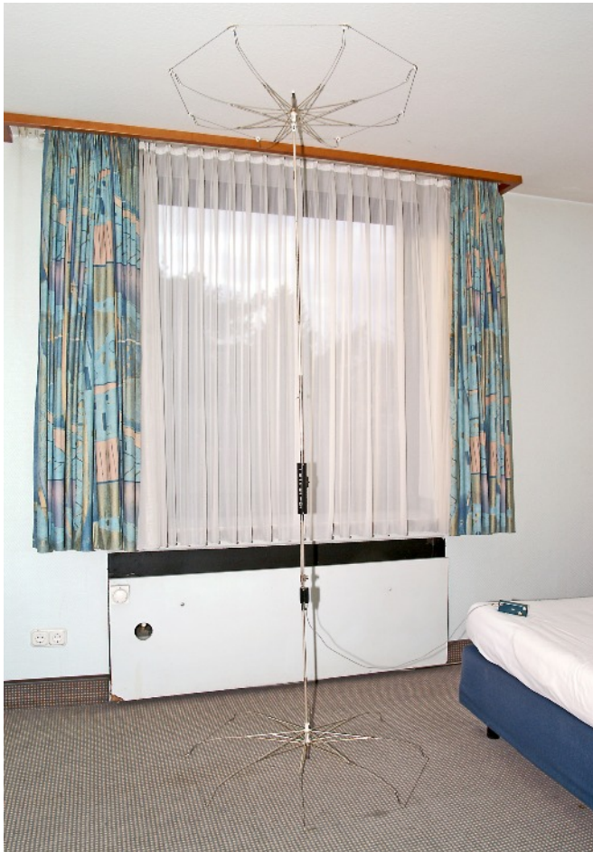
General view of an 'Umbrella' aerial placed in a hotel room, connected to the low-pass filter.
