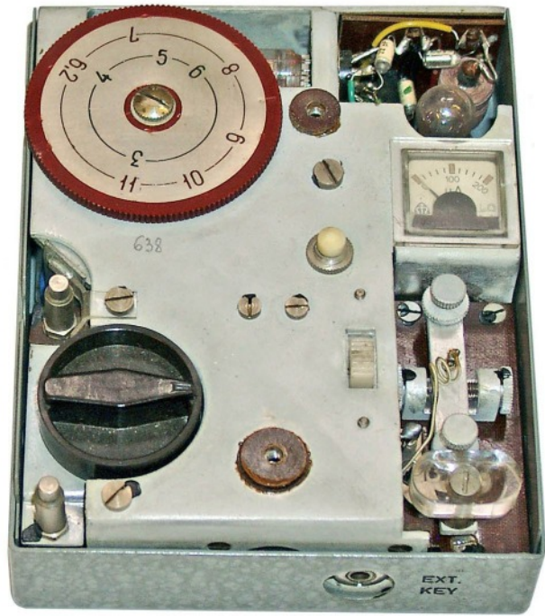
Internal view of Neptun transmitter with top cover removed. Note the miniature hand-speed Morse key in the right hand bottom corner.
