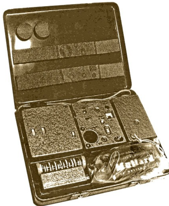
Complete Neptun transmitter with accessories (note the Mullard spare valve wrapped in plastic) packed in a transit case.
