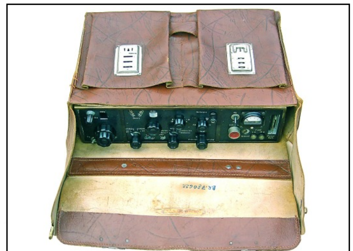
The SEM-78 was packed and carried in an inconspicuously looking leather briefcase. Accessories were stowed in the two compartments on the side of the case.
