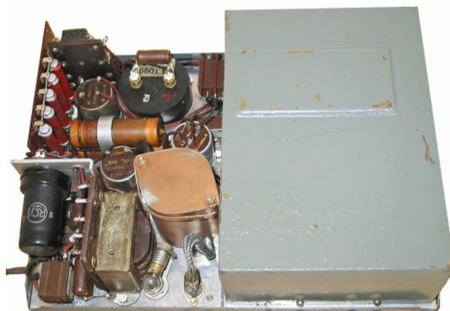
**General view (left) and internal view (above) of the Polish test set. Note that the RF oscillator section and attenuator of the signal generator were enclosed in two fully screened compartments (box at right and cylinder in the centre). The five large resistors (to be seen on top left) were part of the transmitter dummy load.**
